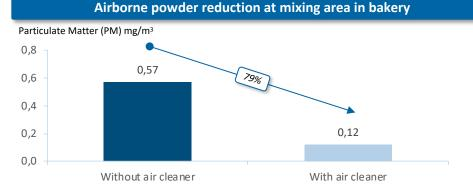
The above graph shows particulate matter measurement after installing a air cleaner at the mixing area in a bakery, resulting in a reduction of particulate matter by 79%
